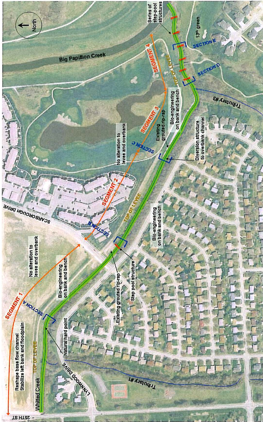
FIGURE 9 Overview of Conceptual Design Whitted Creek Stabilization Study
